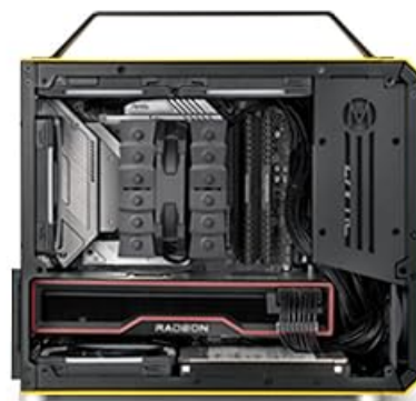
Figure 7: Example build with MATX motherboard and air cooler configuration.
