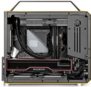
Figure 8: Example build with MATX motherboard and 240 AIO liquid cooling configuration.
