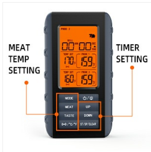
Image: Receiver unit with visible buttons for mode, meat, taste, up, down, and timer controls.
