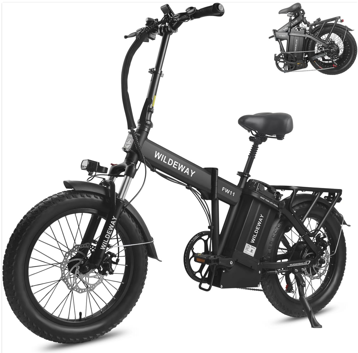
Figure 2.1: The Wildeway FW11 Folding Electric Bike in its unfolded state, showcasing its main features including the fat tires, suspension fork, and rear rack.
