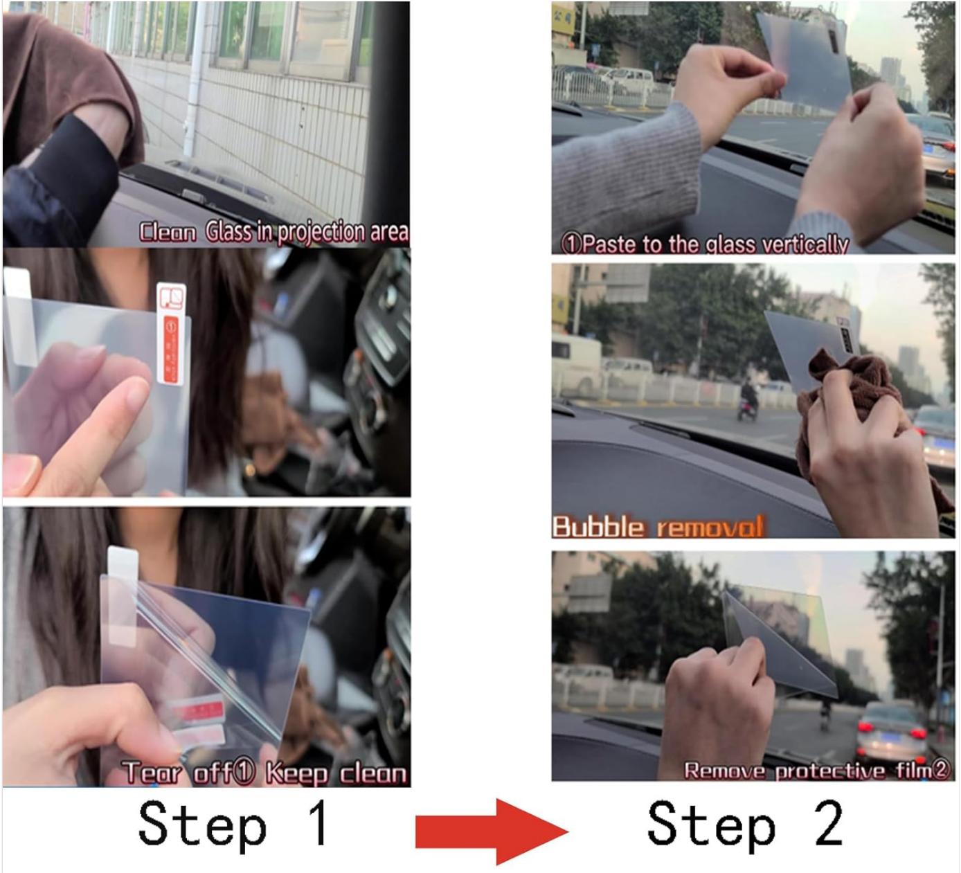
Figure 5: Instructions for applying the reflective film.
