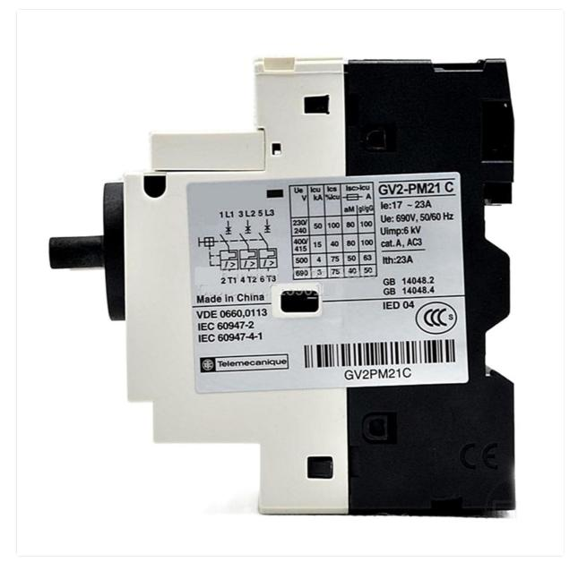
Figure 3.4: Detailed Technical Label. A close-up of the technical label on the side of the breaker, clearly showing the electrical ratings, such as the current adjustment range (le: 17-23A), rated operational voltage (Ue: 690V, 50/60Hz), impulse withstand voltage (Uimp: 6kV), and various breaking capacities (lcs, lcu) at different voltages.
