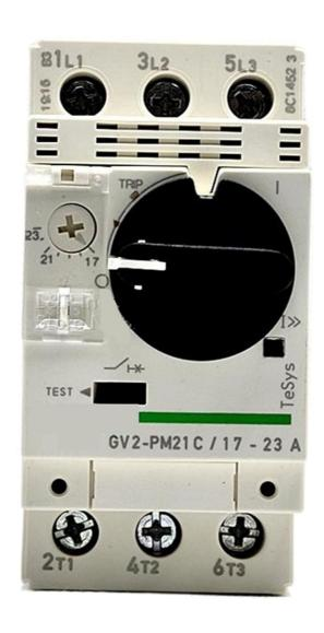
**Figure 3.1: Front View of GV2-PM21C.** This image displays the front of the motor circuit breaker, showing the rotary knob for operation, the 'TRIP' indicator, the 'TEST' button, and the main power terminals (1L1, 3L2, 5L3 at the top; 2T1, 4T2, 6T3 at the bottom).
