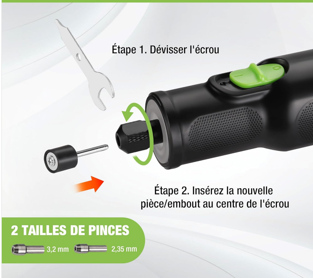
Figure 5: Two-step accessory replacement process.
