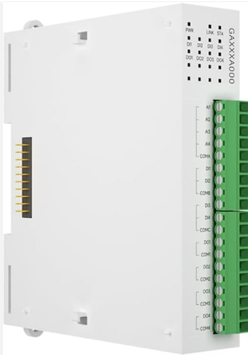
Figure 1: CDBAIRUI GAXAX8080 Distributed Remote IO Expansion Module, front view showing indicators and terminal blocks.
