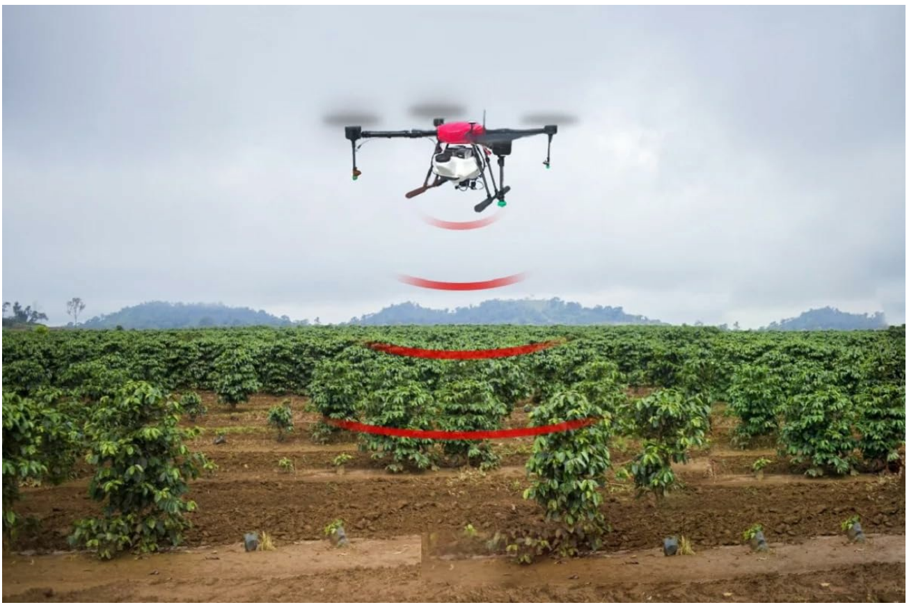
Figure 6: A close-up illustration of the NRA24 altimeter's radar beam interacting with the ground, ensuring precise altitude control for drone operations.
