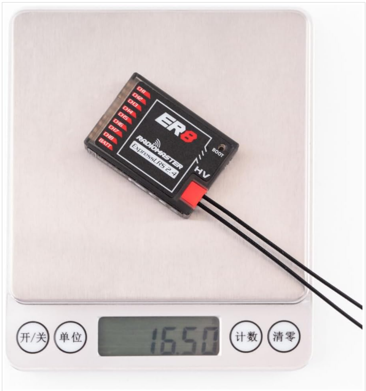
Image 3.2: The RadioMaster ER8 receiver on a digital scale, displaying a weight of 16.50 grams.
