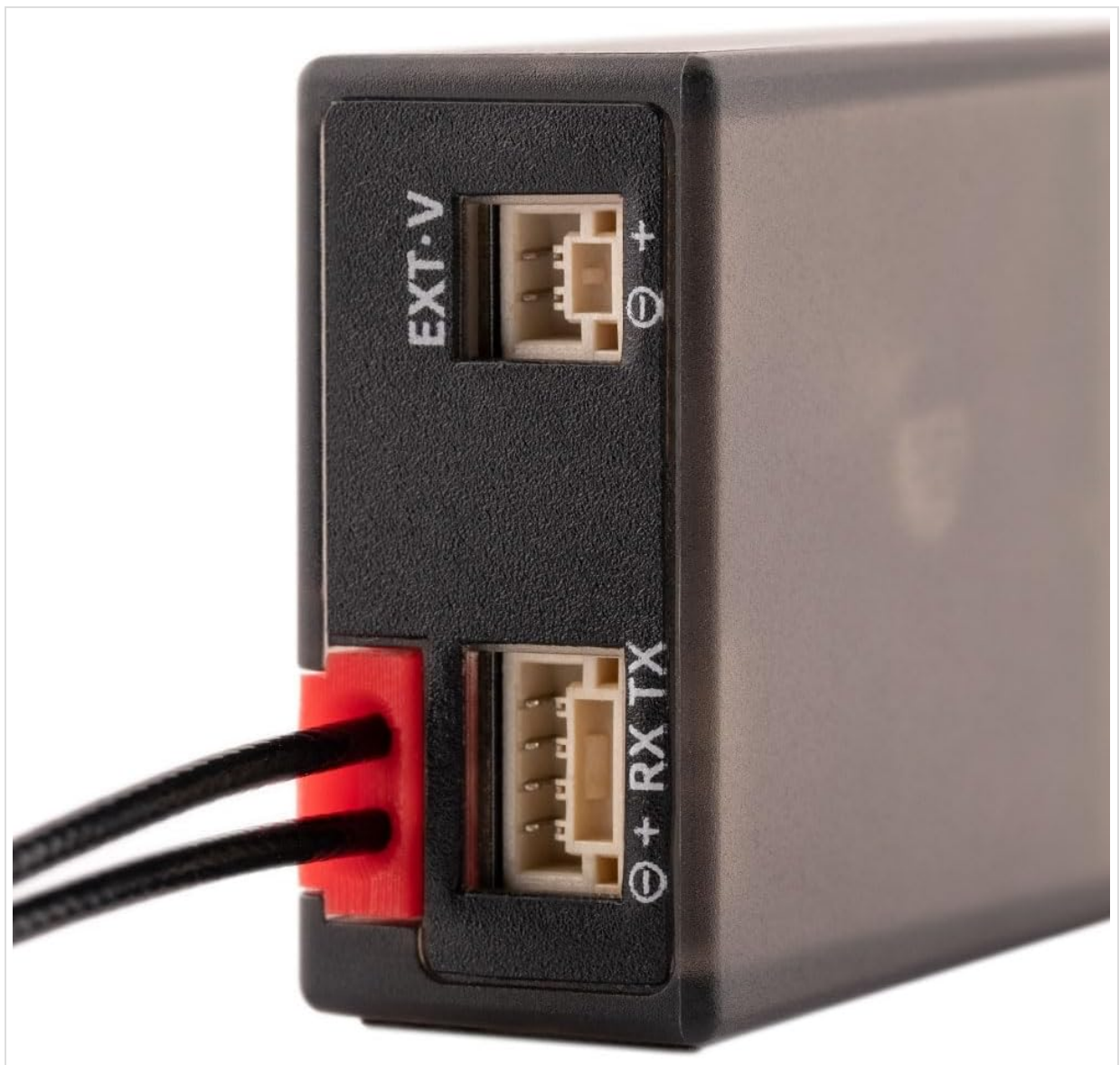
Image 5.1: Side view of the ER8 receiver showing the EXT-V port for external voltage telemetry and the + RX TX port for CRSF bus interface connections.
