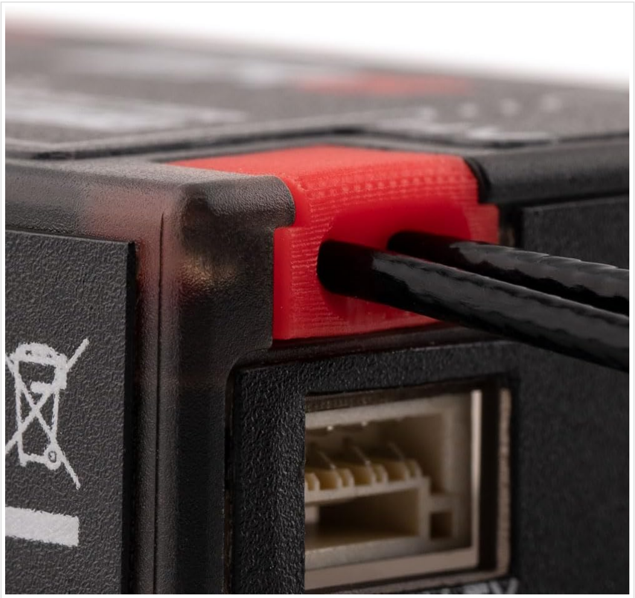
Image 5.2: Close-up of the ER8 receiver's antenna connection points and the 'BOOT' button, which is used for firmware updates and binding.
