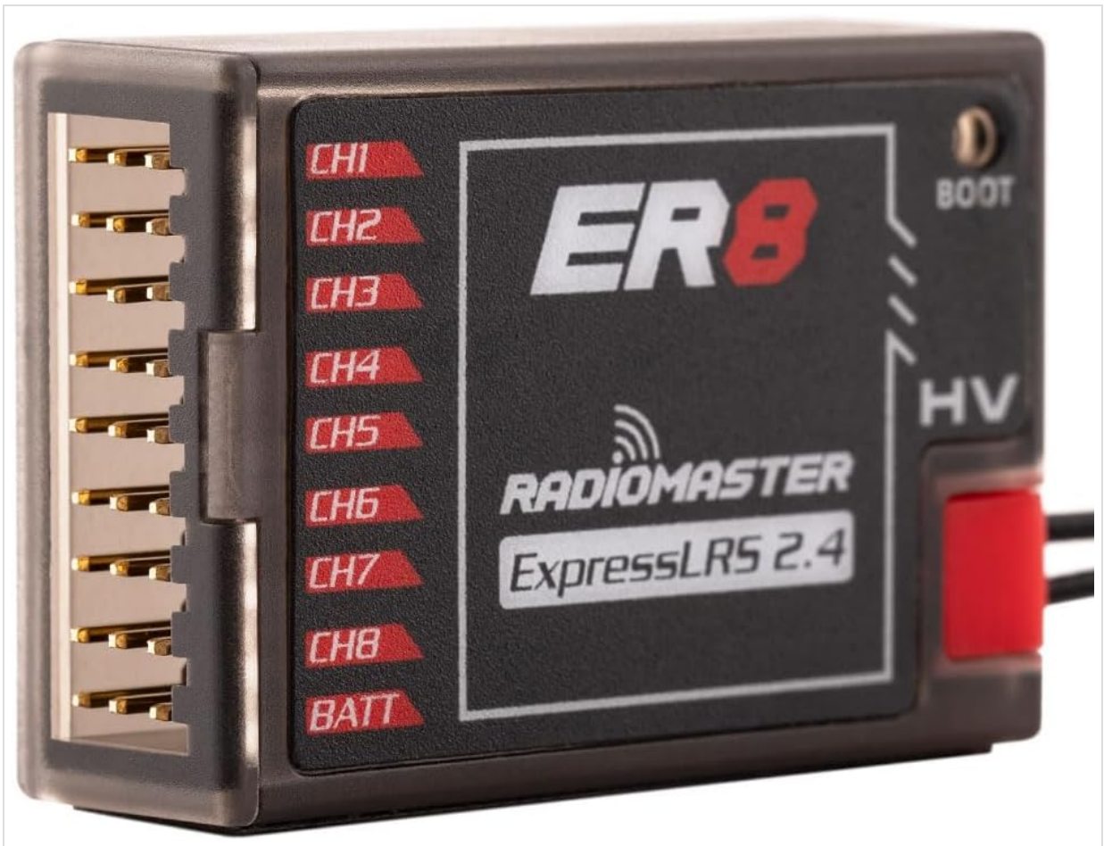
Image 2.1: Front view of the RadioMaster ER8 receiver, showing the 8 PWM output channels and the ExpressLRS 2.4 branding.
