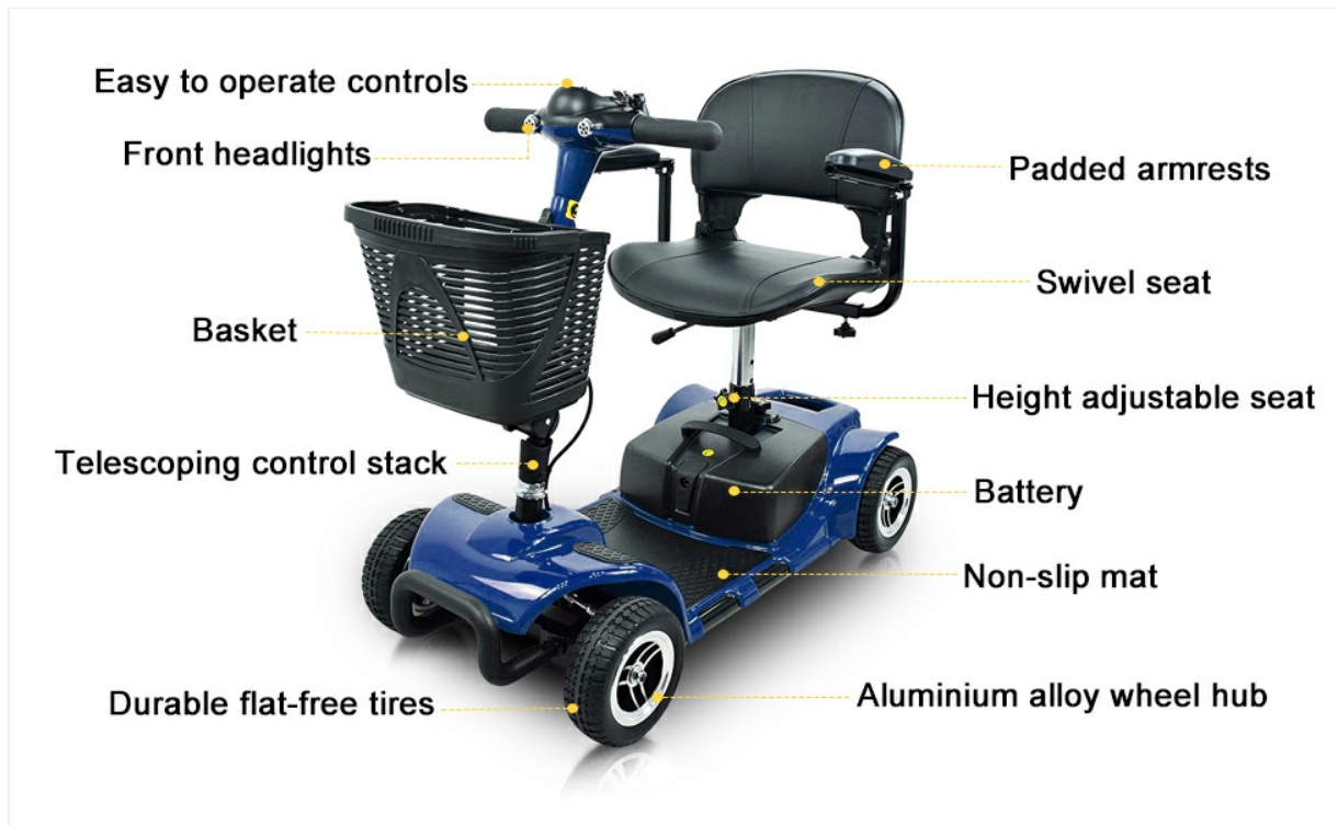
Figure 3.1: Labeled components of the E-MOTOR Mobility Scooter.
