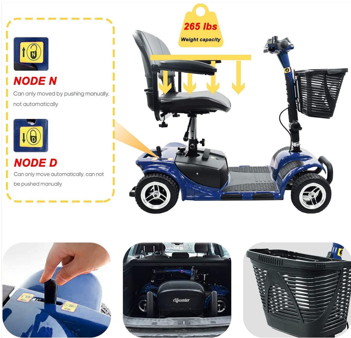
Figure 2.2: Scooter components and an example of storage in a car trunk.
