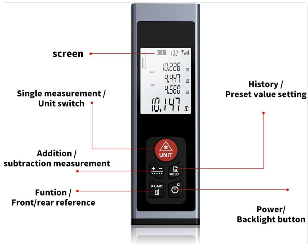
Figure 2: Device Components and Controls
