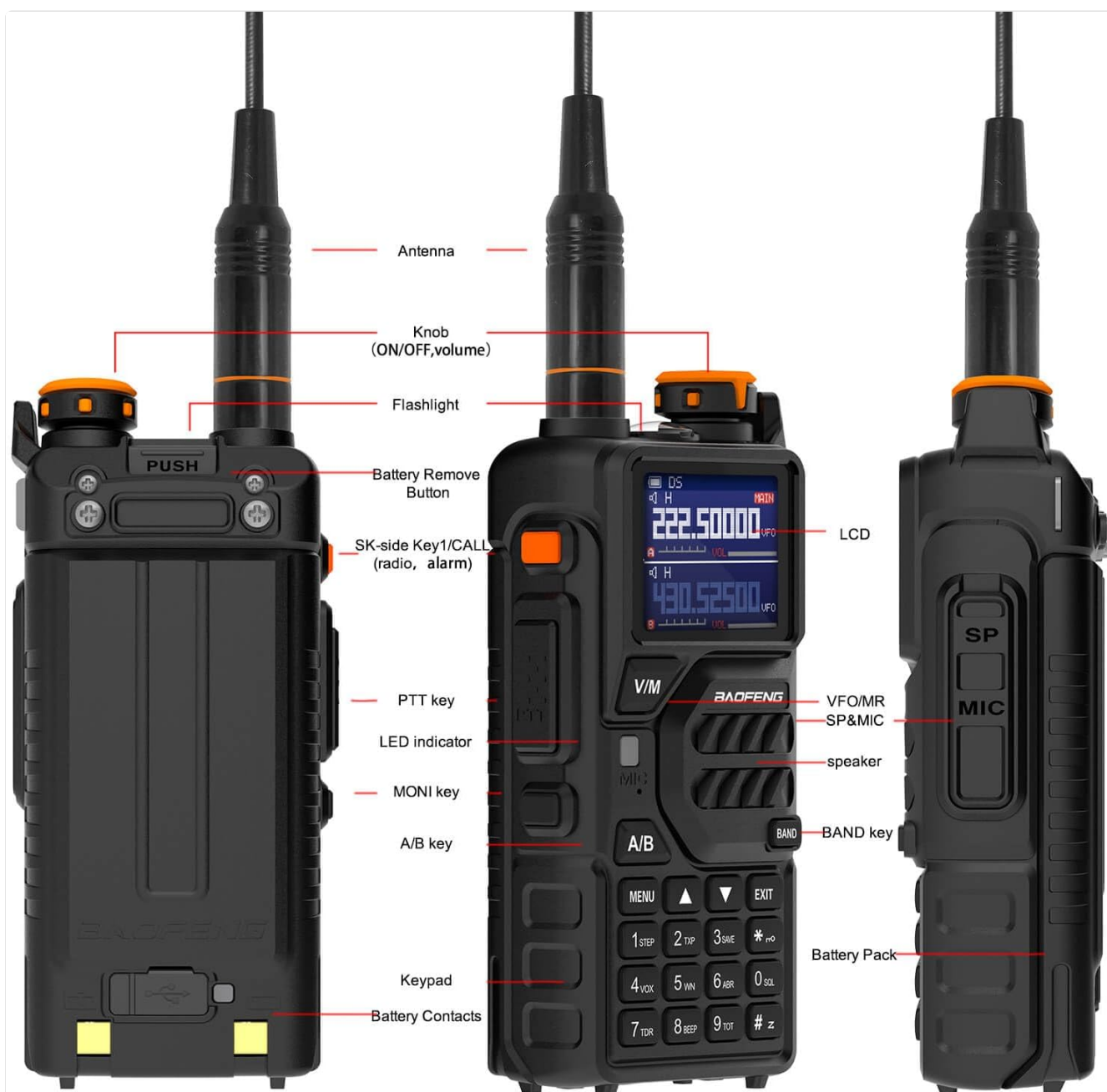
Figure 3.1: Labeled diagram of the BAOFENG K5PLUS radio, highlighting the antenna, knob (ON/OFF/volume), flashlight, battery remove button, SK-side Key1 (radio, alarm), PTT key, LED indicator, MONI key, A/B key, keypad, battery contacts, LCD, VFO/MR, SP&MIC, speaker, BAND key, and Battery Pack.
