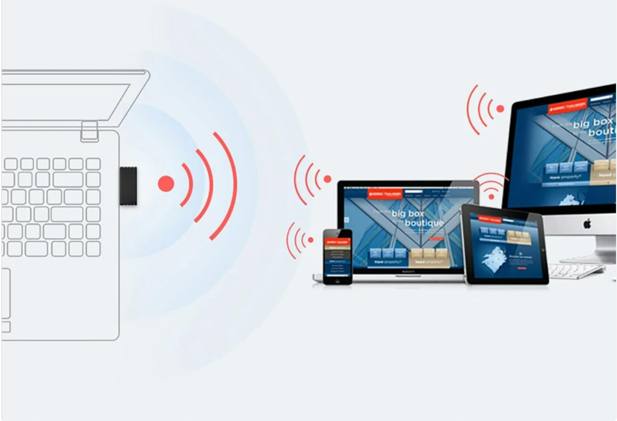
Image: A diagram illustrating the Soft AP function, where a laptop with the USB WiFi adapter shares its internet connection, allowing other devices like phones and other computers to connect wirelessly.
