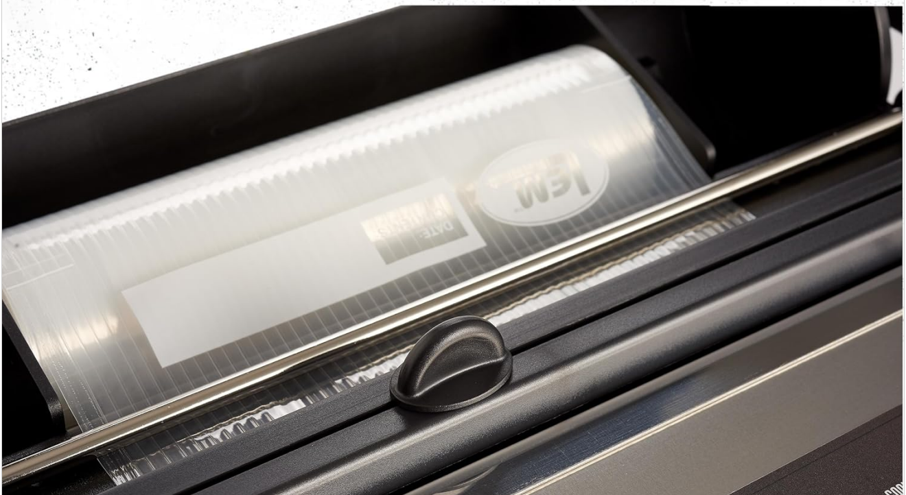
Figure 4: Preparing a custom-sized bag using the integrated roll holder and cutter.
