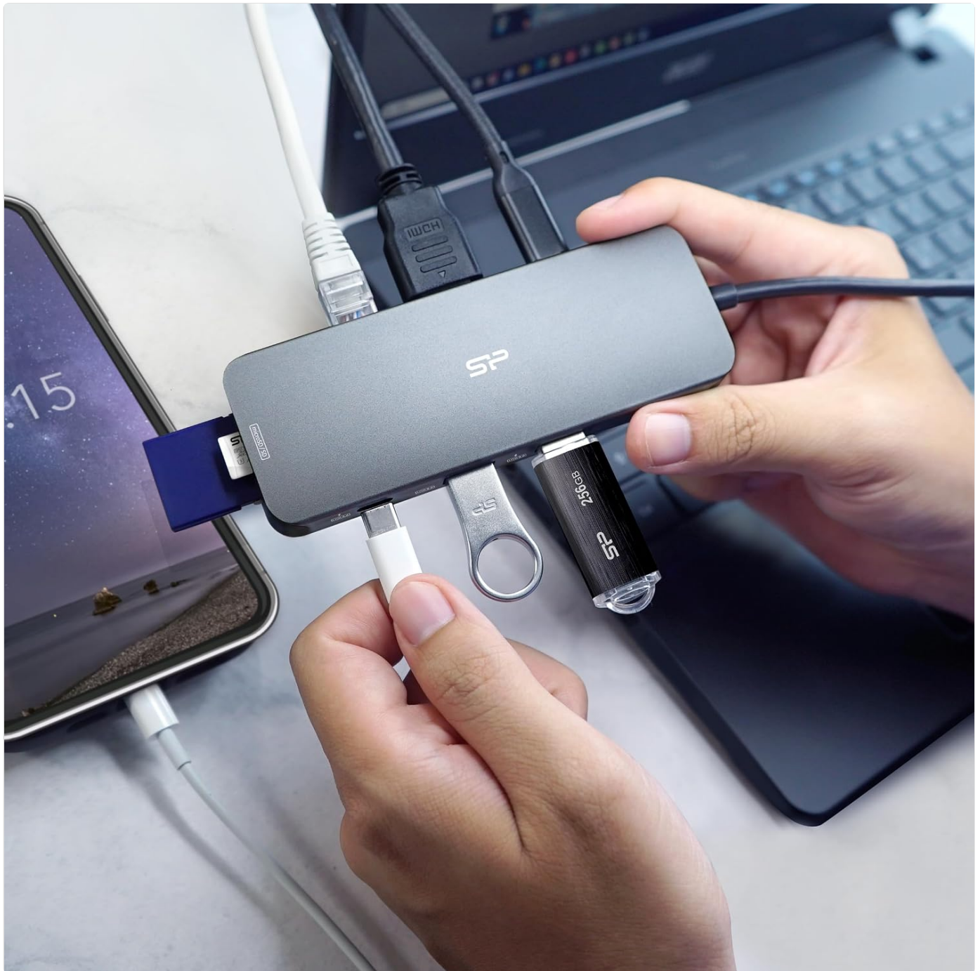
Figure 3: A user connecting various devices to the SR30 docking station, including USB drives and an SD card.
