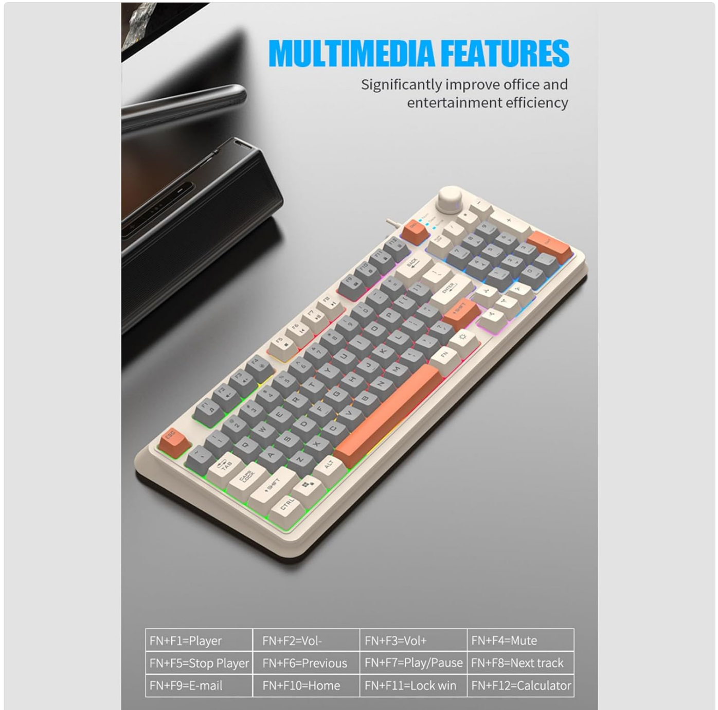
Image 4.1: The 94-key minimalist layout of the K82 keyboard, highlighting its space-saving design compared to a standard 104-key layout, and demonstrating mixed color lighting effects.
