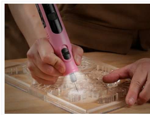
Image: A person using the WORKPRO rotary tool with a carving bit to engrave a design onto a clear acrylic sheet, demonstrating its precision for detailed work.
