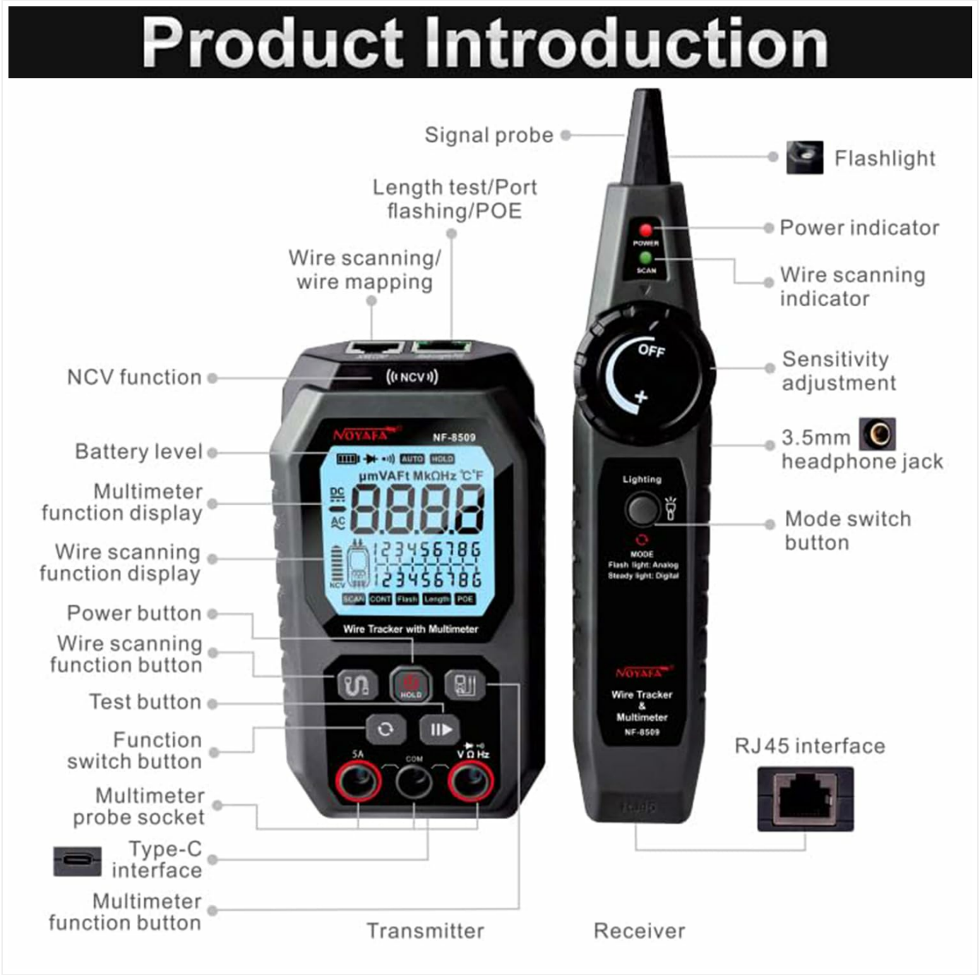
Image 2.1: Diagram illustrating the various buttons, ports, and display elements on both the transmitter and receiver units of the NF-8509.
