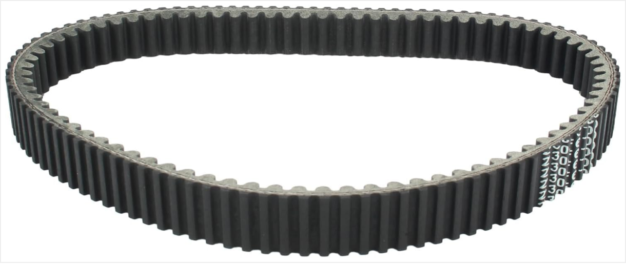
A continuous variable transmission (CVT) drive clutch belt, black with ribbed inner and outer surfaces, designed for power transfer in UTV and ATV applications.
