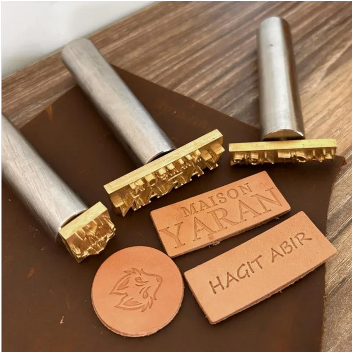
Image: A collection of custom leather stamps and their corresponding handles, alongside examples of stamped leather.
