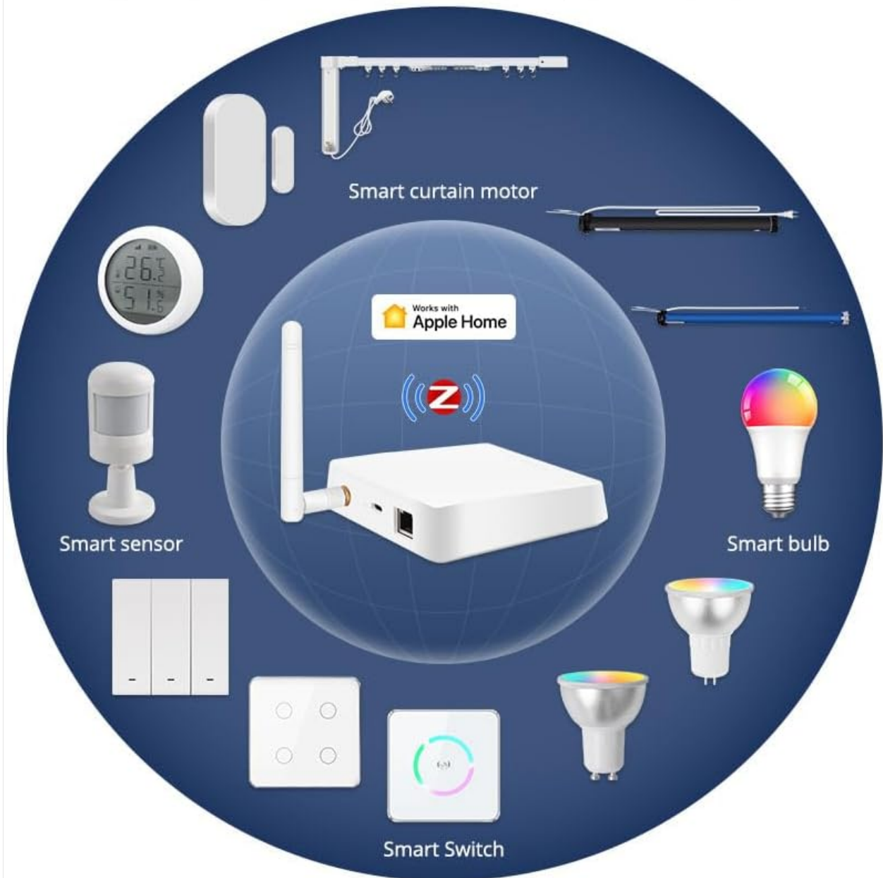
Image 3.1: A diagram illustrating the Zigbee Hub as a central bridge connecting various smart home devices such as smart curtain motors, sensors, bulbs, and switches within an Apple Home environment.
