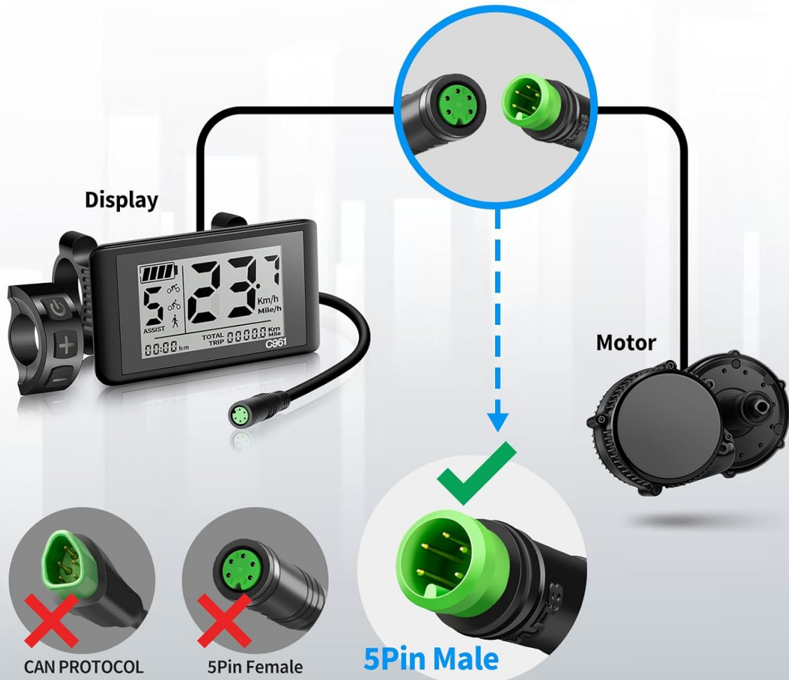
Figure 2: Compatibility Diagram. This diagram shows that the C961 display requires a 5-pin male connector on the motor for proper connection. It explicitly states incompatibility with CAN protocol and 5-pin female motor connectors.
