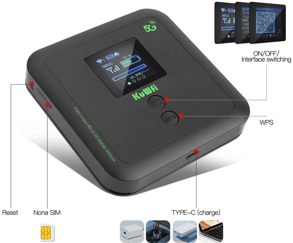
Image: Detailed view of the KuWFi 5G01 device, highlighting its various ports and buttons.
