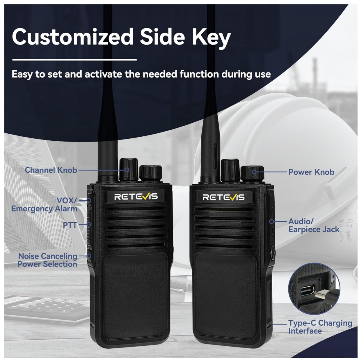
Image: Labeled diagram of the Retevis P2 radio's controls and ports.
