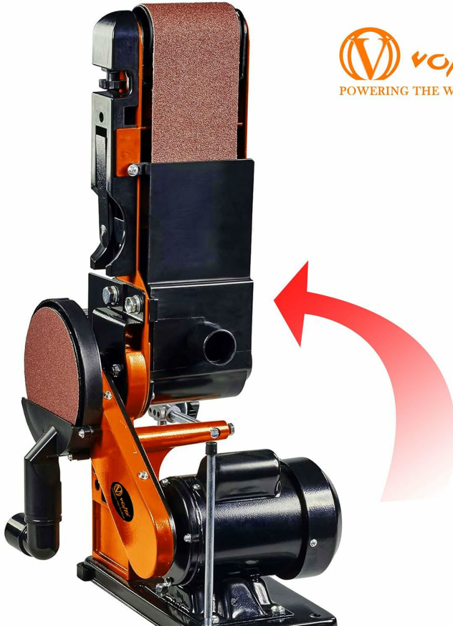
Figure 5.1: The sanding belt can be adjusted to a vertical position for specific tasks.
