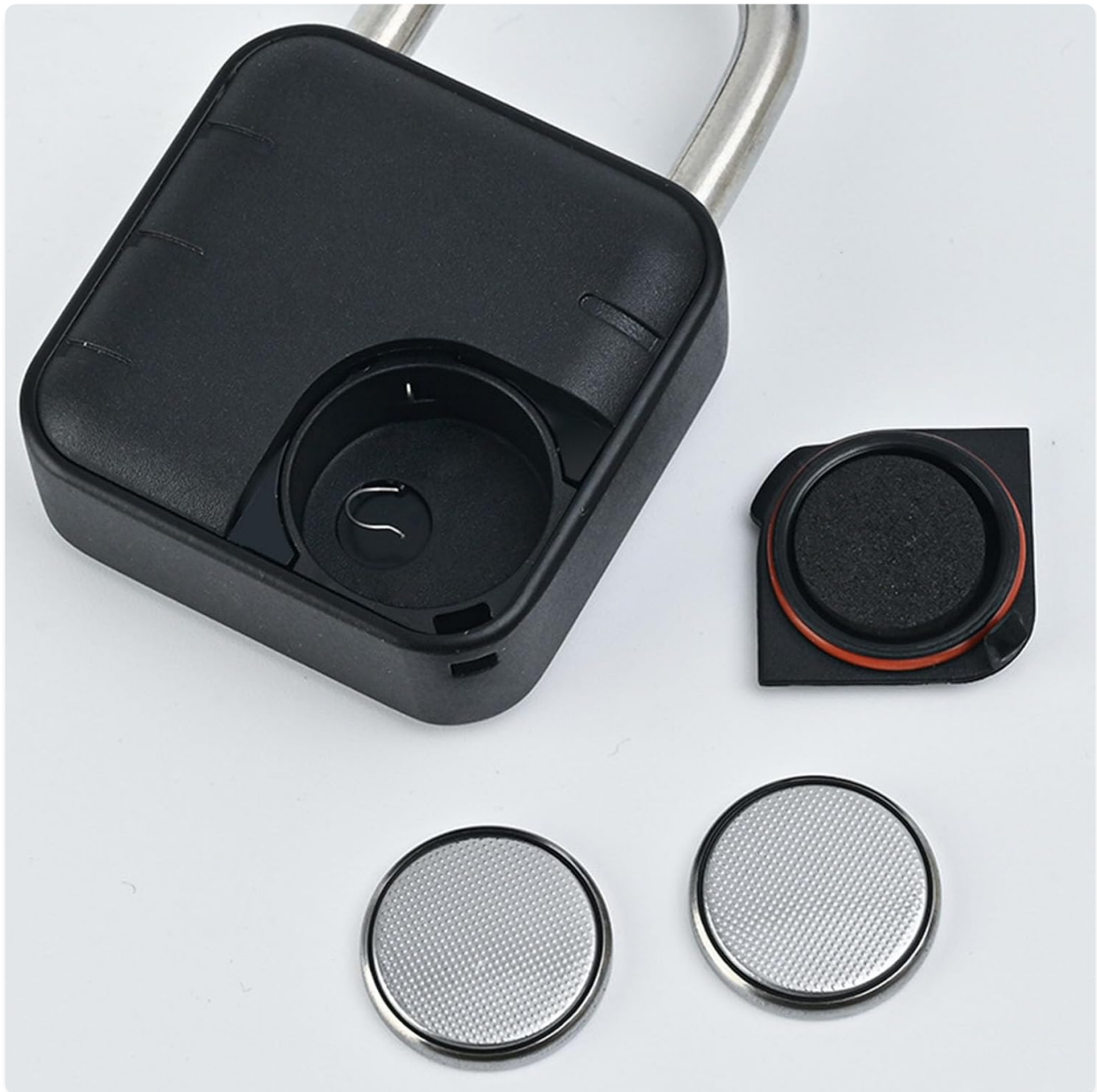
Figure 2: View of the battery compartment, showing where the plastic film needs to be removed.
