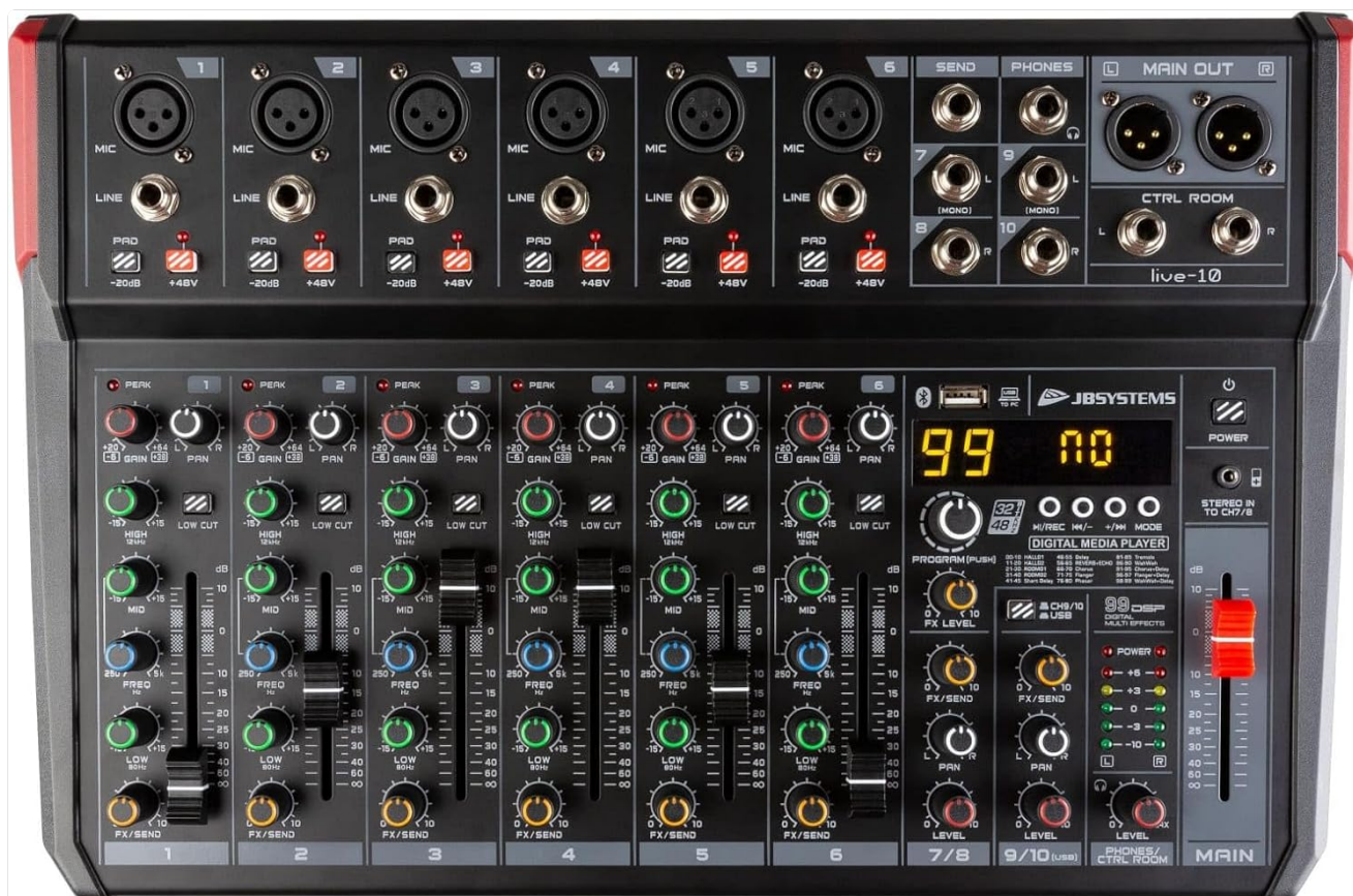
Image 4.1: Front panel of the JB systems LIVE-10 mixer, showing all input channels, controls, and the media player section.
