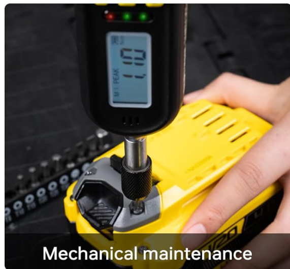
Figure 3: Switching between Track and Peak modes.
