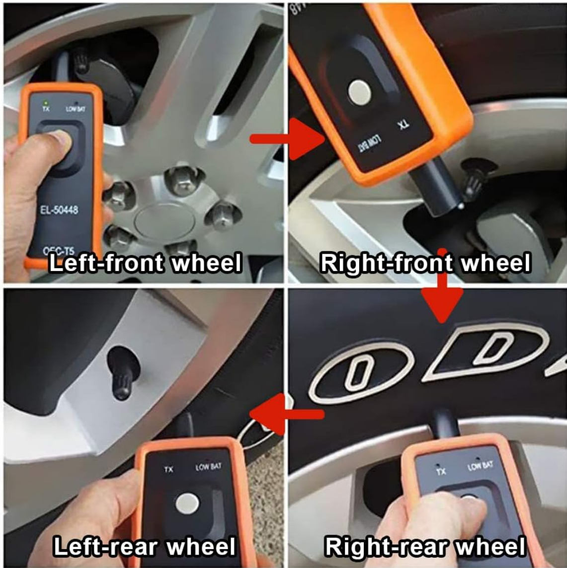
Figure 5: Application display. This image shows the tool being used on each of the four wheels (left-front, right-front, left-rear, right-rear) during the TPMS relearn process.
