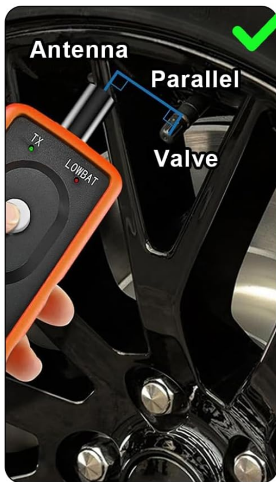
The best location for the antenna
