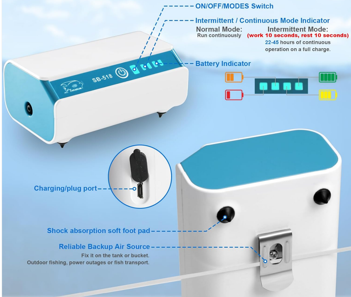
Image: Product details highlighting the ON/OFF/MODES switch, battery indicator, charging/plug port, shock absorption soft foot pads, and reliable backup air source metal clip.
