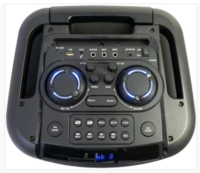
This top-down view details the control panel of the Ibiza MOBILE800. It features various rotary knobs for adjusting volume, bass, treble, echo, and delay. Below these, a row of buttons provides control for mode selection, track navigation (previous, next), play/pause, record, TWS pairing, X-Bass activation, and LED lighting modes. Input ports for TF card, USB, AUX, Guitar, and two Microphones (MIC1, MIC2) are clearly labeled, along with the DC 15V power input and the main power switch (ON/OFF).
