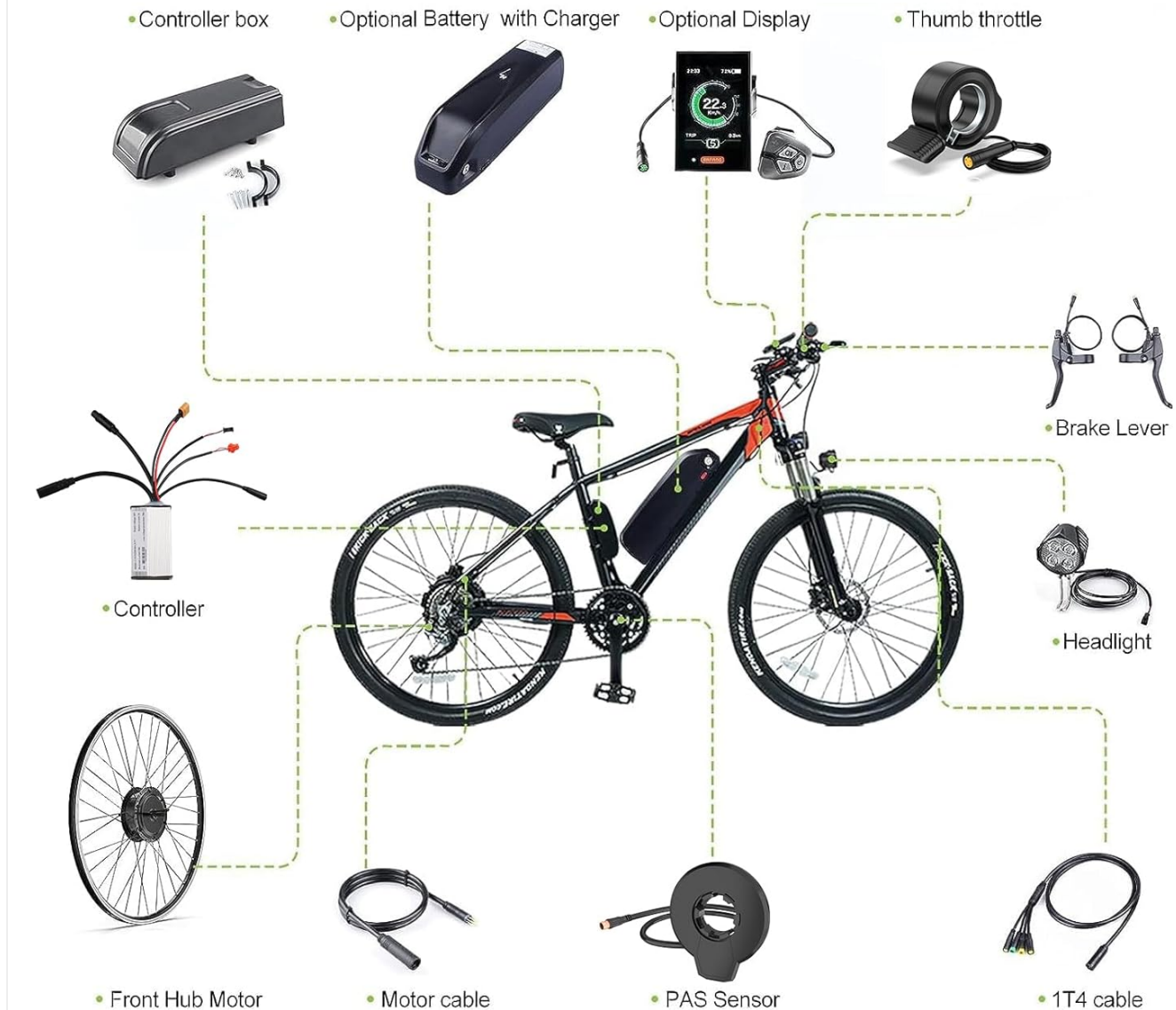
Figure 4.1: Kit Connection Diagram.
