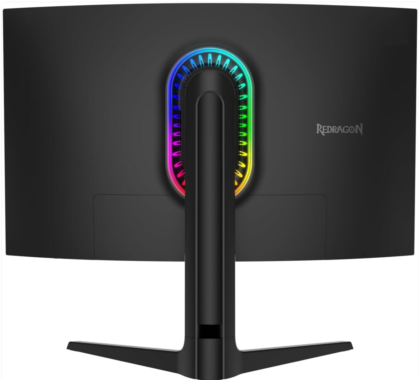
Figure 5.1: Rear view of the Redragon Tassos GM32H2Q monitor, showcasing the integrated RGB lighting around the stand attachment point. This lighting can be customized or turned off via the OSD menu.
