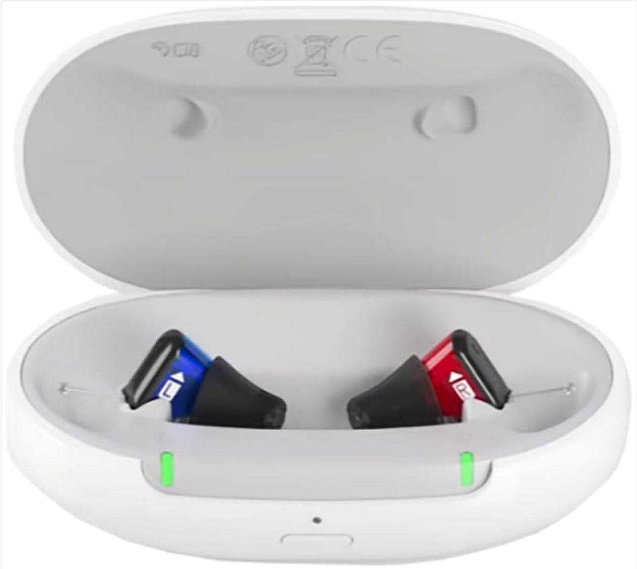
Image 3: The Signia Silk Charge & Go IX portable charger with two Signia Silk IX hearing aids correctly placed in their respective charging slots. Green indicator lights are visible, signifying that the hearing aids are actively charging.
