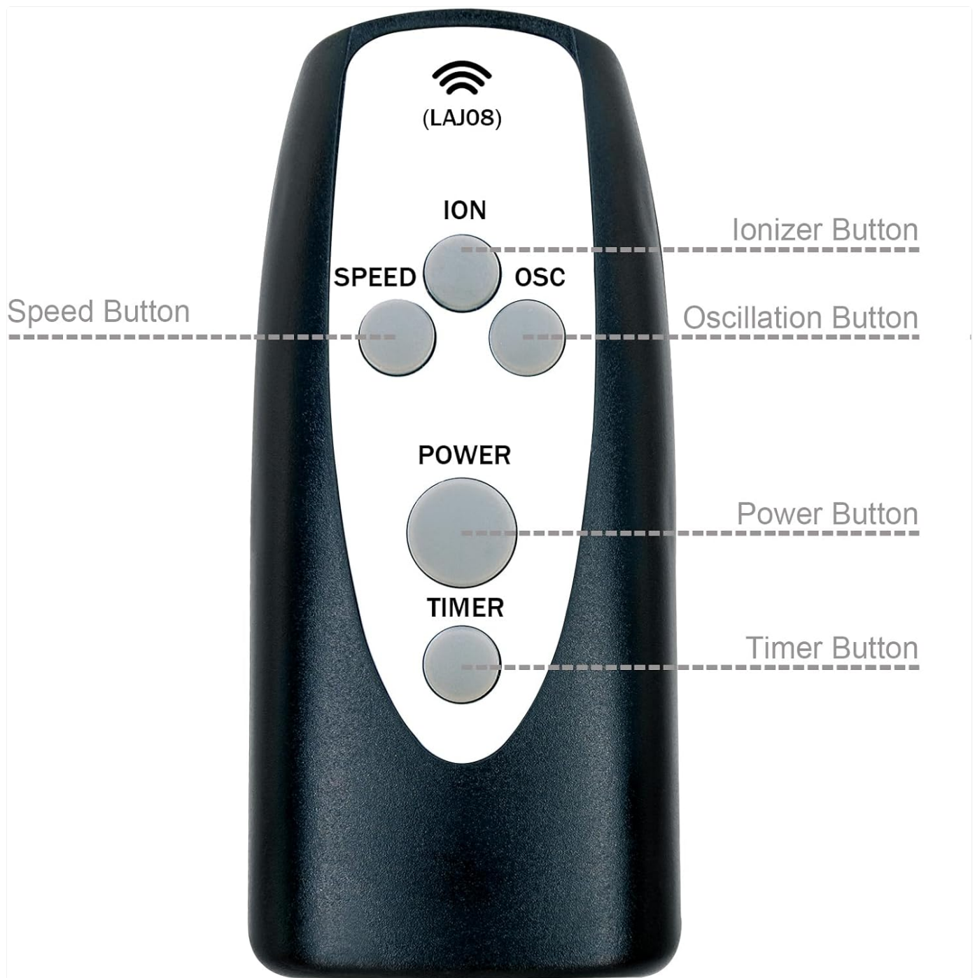
Image: A detailed diagram of the remote control, clearly labeling each button and its corresponding function: Ionizer Button, Speed Button, Oscillation Button, Power Button, and Timer Button.
