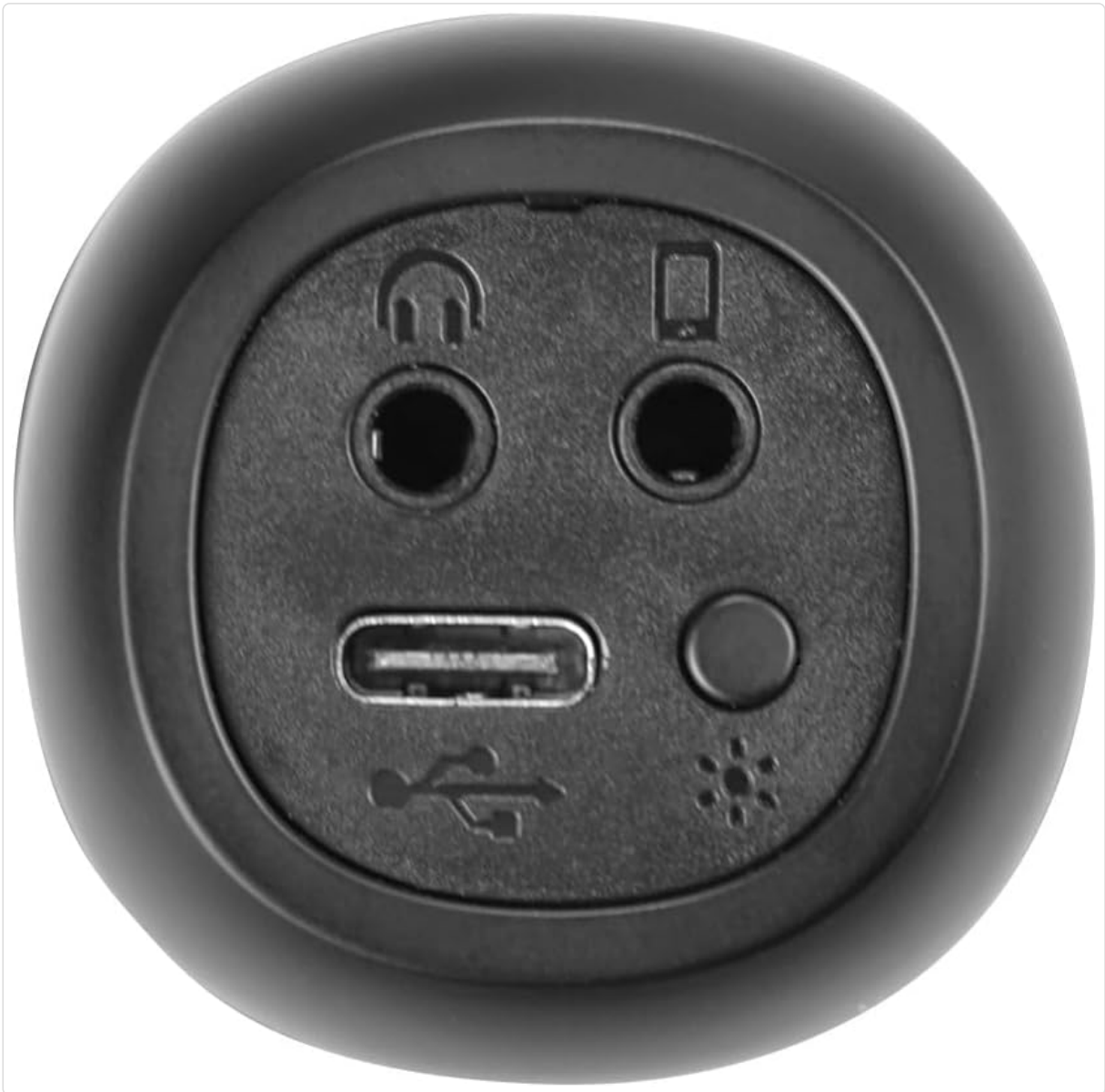
Image: Close-up view of the bottom of the microphone, showing the USB-C charging port, 3.5mm audio input/output jacks, and the light mode button.
