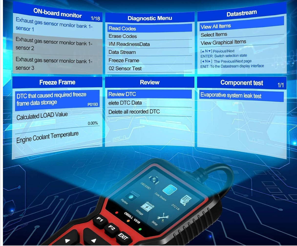
Figure 6: The V519's on-screen interface, showing examples of the Diagnostic Menu (Read Codes, Erase Codes, I/M Readiness, Data Stream, Freeze Frame, O2 Sensor Test) and a Datastream view with graphical items.
