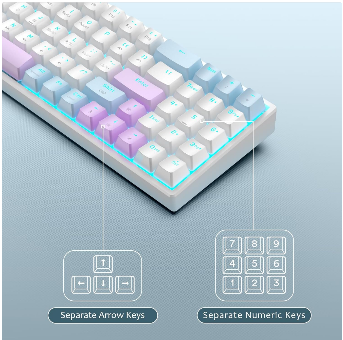
Figure 6: Separate Arrow and Numeric Keys. This image highlights the dedicated arrow keys and the integrated numeric keypad functionality, accessible through specific key combinations on the compact keyboard layout.
