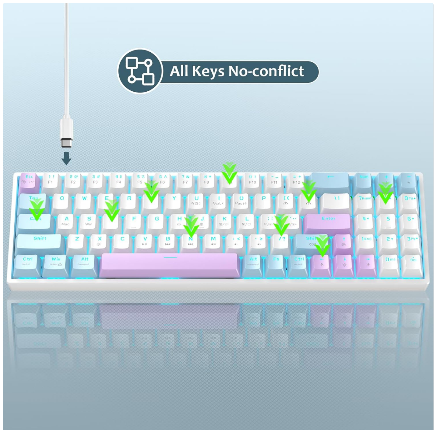
Figure 7: All Keys No-conflict Feature. This image visually represents the N-key rollover capability, indicating that all key presses are registered simultaneously without conflict, which is beneficial for fast typing and gaming.
