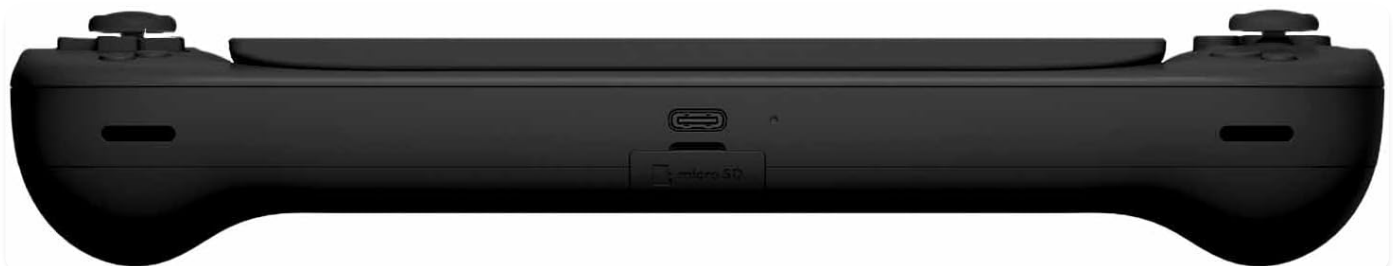
Bottom view of the AYA NEO Slide, revealing the second USB4 Type-C port and the Micro SD card slot.
