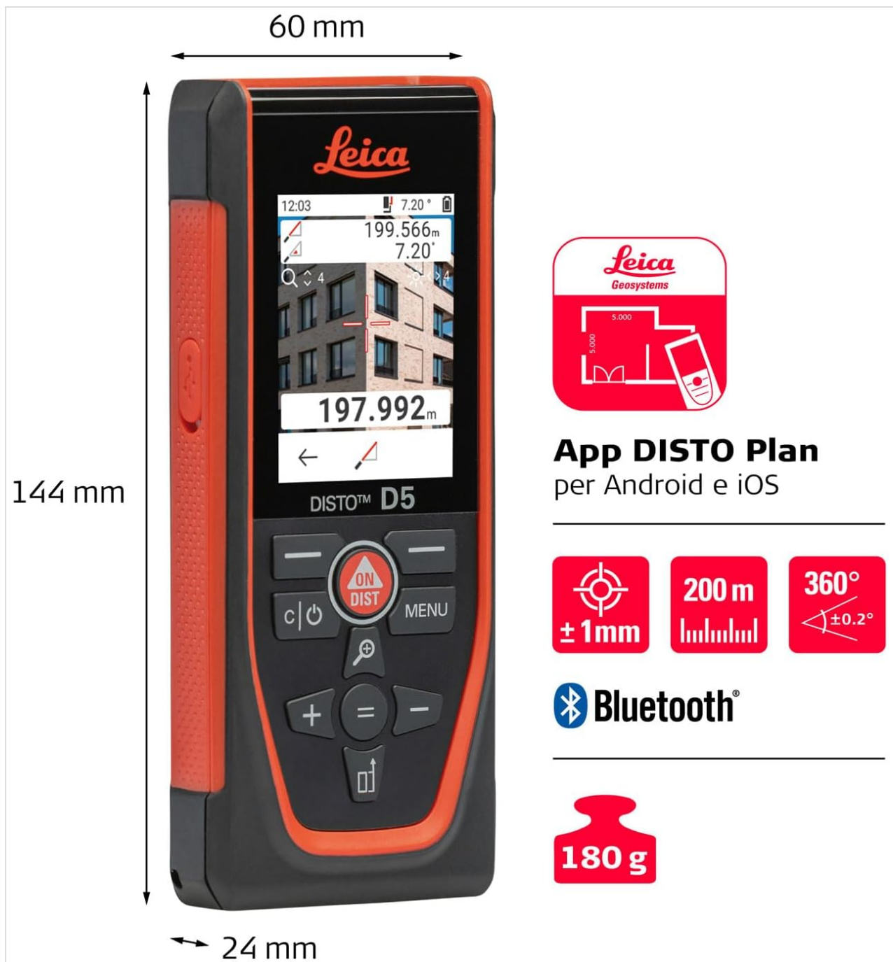
Image 9.1: Visual summary of Leica Disto D5 specifications, including range, accuracy, inclinometer, Bluetooth, and weight.
