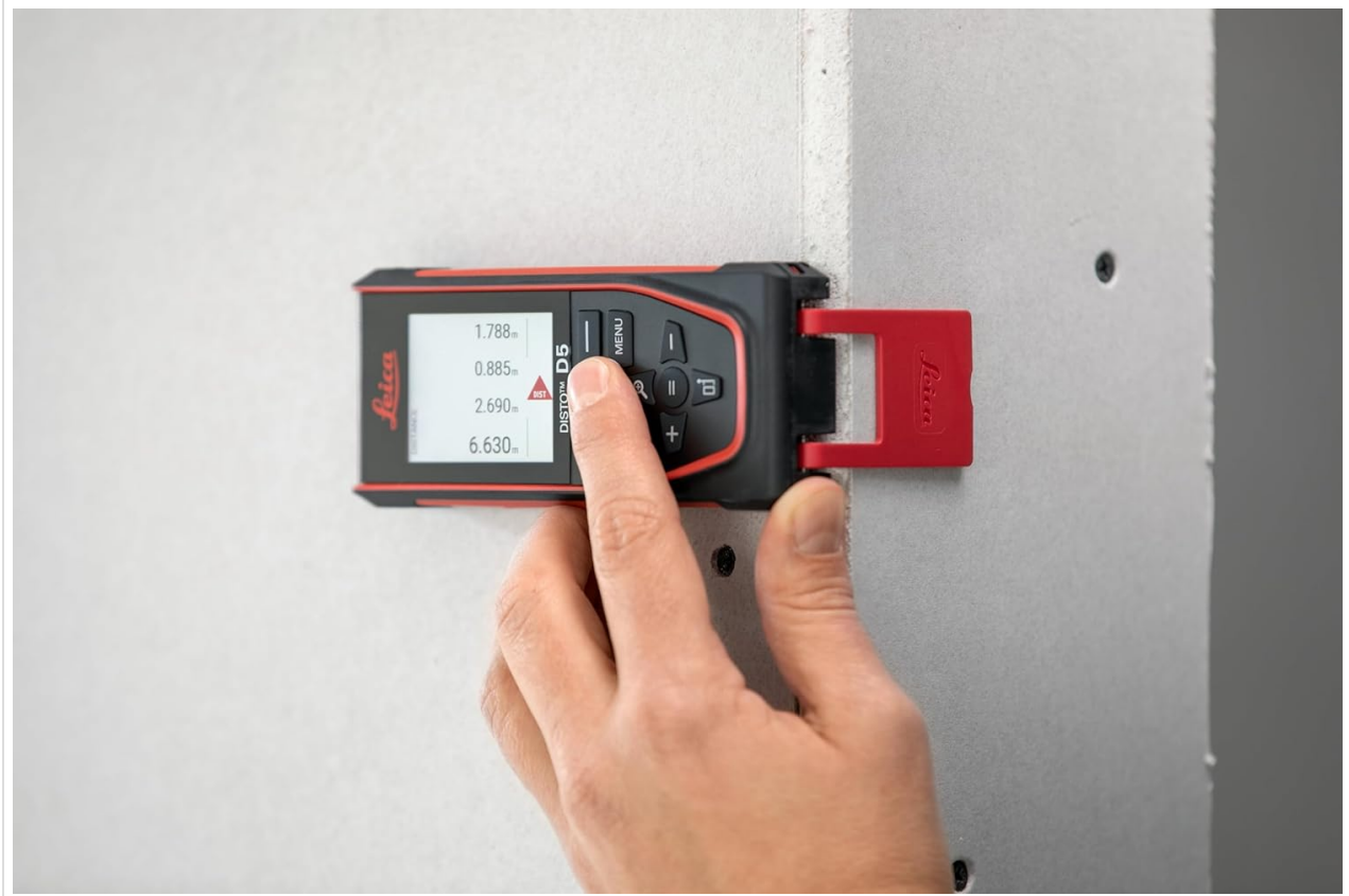
Image 6.1: Performing a basic distance measurement with the Leica Disto D5, showing the device held against a surface.
