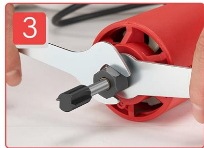
3 Tighten the collet with wrenches
