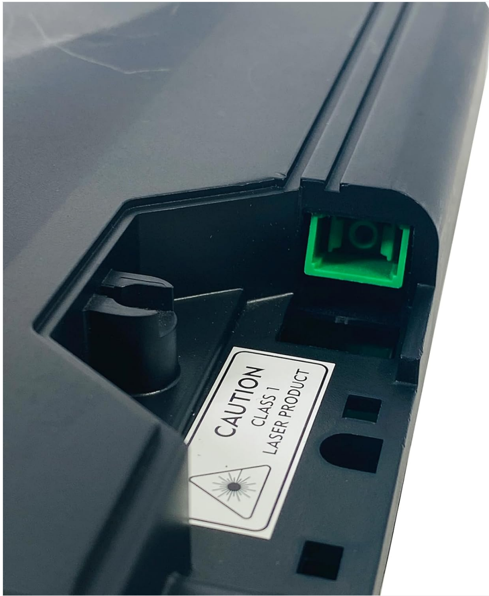
Figure 2: Optical port with Class 1 Laser Product warning label.
