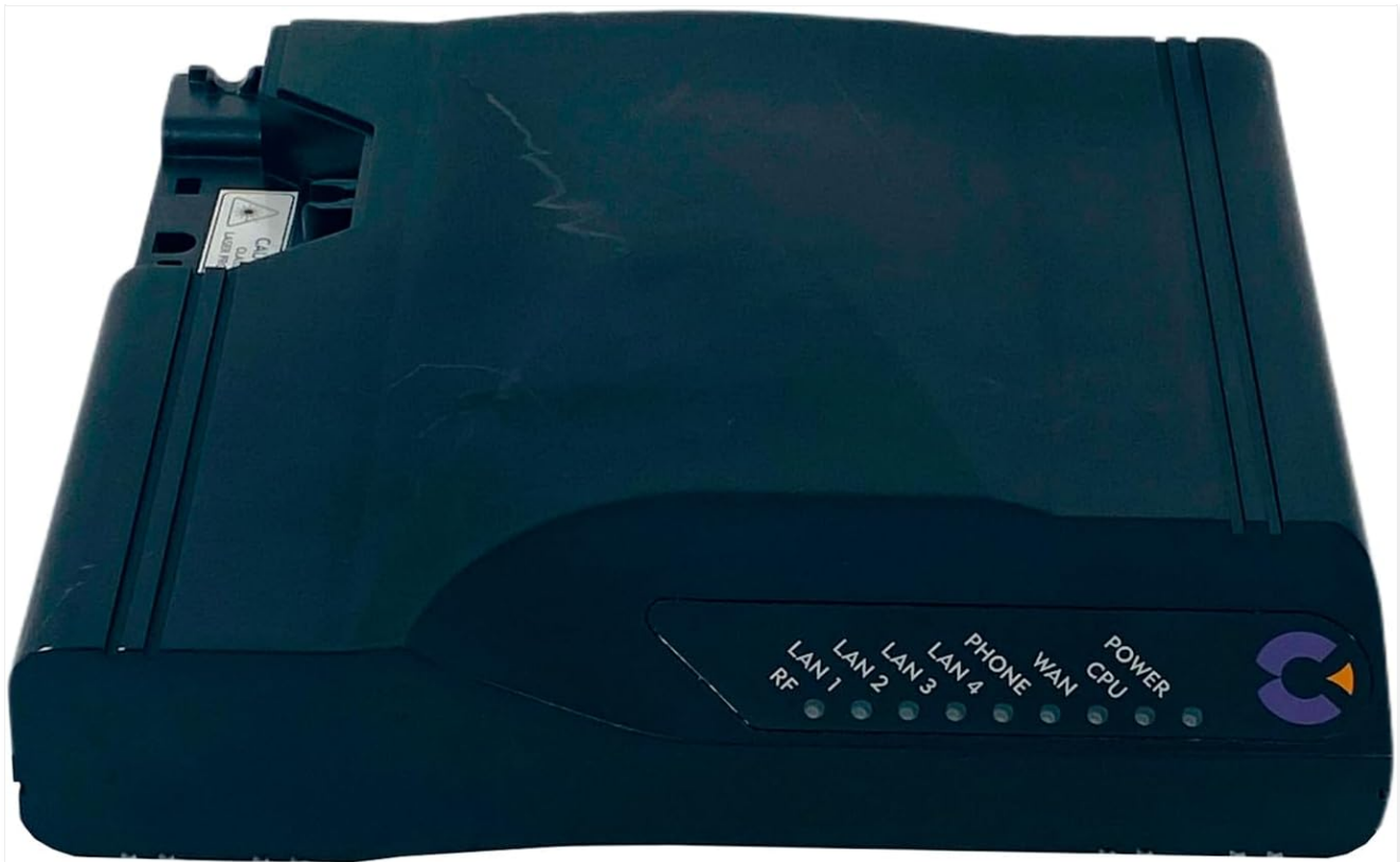
Figure 3: Front panel LED indicators.
