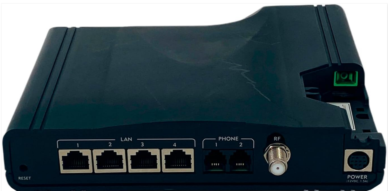
Figure 4: Rear panel connectivity ports.
