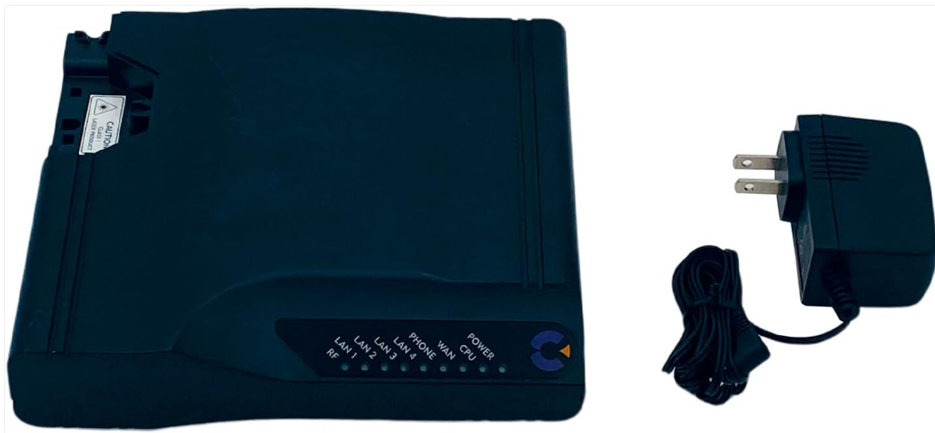
Figure 1: Calix 726GE-I ONT with included AC power adapter.
