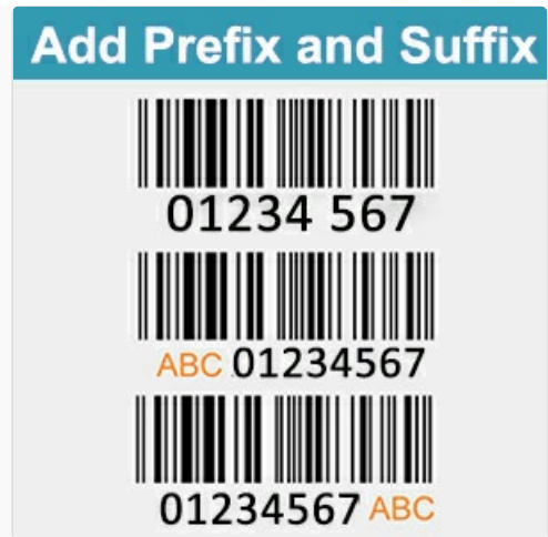
Image 4.4: Visual representation of adding a prefix (e.g., 'ABC') or suffix to scanned barcode data.
