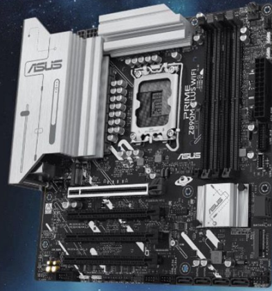
Image: An overview diagram of the ASUS Prime Z890M-PLUS WiFi motherboard, highlighting the LGA 1851 socket, DDR5 DIMM slots, PCIe 5.0 x16 SafeSlot, and M.2 slots.
