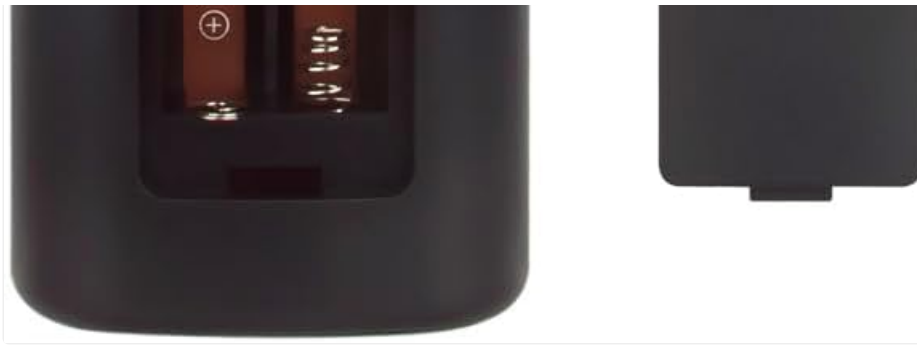
Figure 2: Rear view of the remote control showing the open battery compartment and two AAA batteries. This illustrates the correct orientation for battery insertion.
