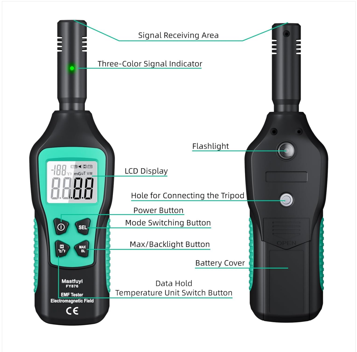
Figure 3.1: Labeled diagram of the Mastfuyi FY876 Digital EMF Tester components.
