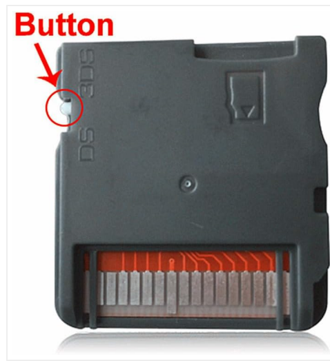
Figure 3: Location of the mode switch on the Ace3ds X cartridge.
