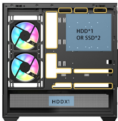
Figure 3.3.1: Diagram showing the locations for 2.5" SSDs (motherboard side) and 3.5" HDDs (bottom and motherboard side) within the SAMA SV02 case, highlighting backplug motherboard support.
