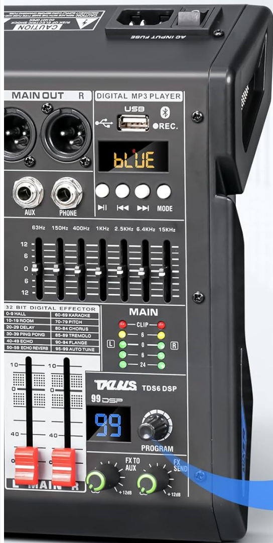
Figure 4.2.1: A visual guide to selecting DSP effects on the TKLBS TDS-6DSP mixer. The display shows the effect number (01-99), and a rotary knob is used to select the effect type, which is then confirmed by pressing the knob. A list of effect categories (Hall, Room, Delay, Ping Pong, Echo, Echo Reverb, Karaoke, Pitch, Chorus, Tremolo, Flange, Auto Tune) is also shown.
