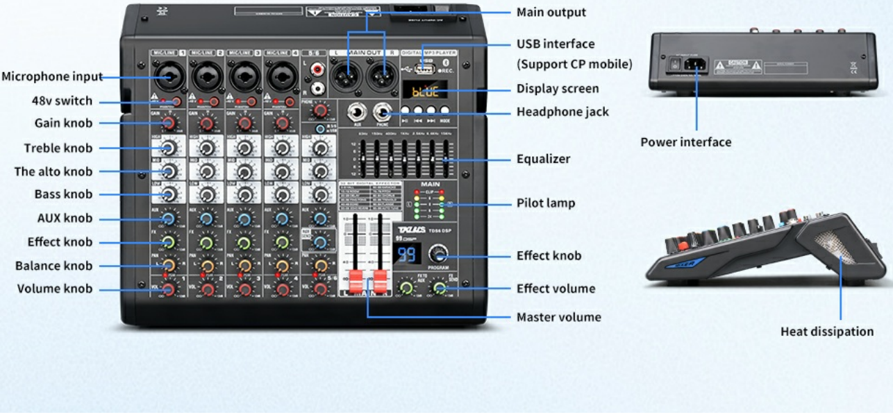
Figure 2.2.1: Front and side view of the TKLBS TDS-6DSP mixer with labels for all inputs, outputs, and controls, including microphone inputs, 48V switches, gain knobs, EQ knobs, AUX knobs, effect knobs, pan, volume faders, main output, USB interface, display screen, headphone jack, equalizer, pilot lamp, effect volume, master volume, power interface, and heat dissipation vents.
