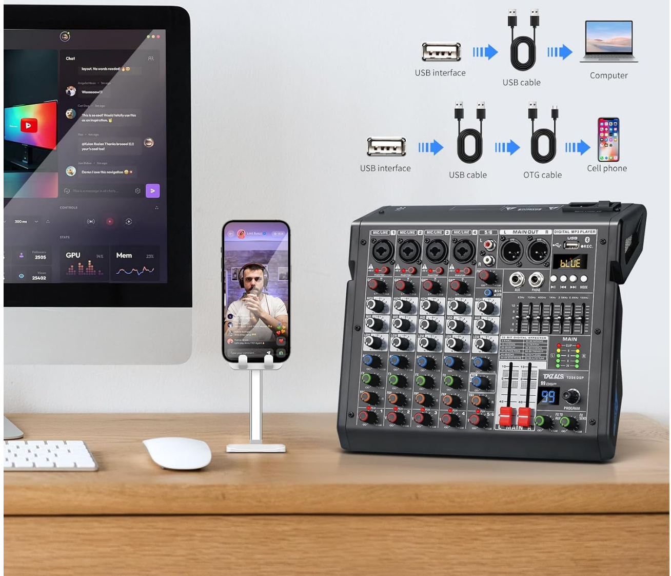
Figure 5.2.1: This image illustrates the mixer's capability as a live recording sound card, supporting PC and mobile lossless transmission. It shows connections via USB-B to a computer and via USB-B with an OTG cable to a cell phone for recording and live broadcasting.
