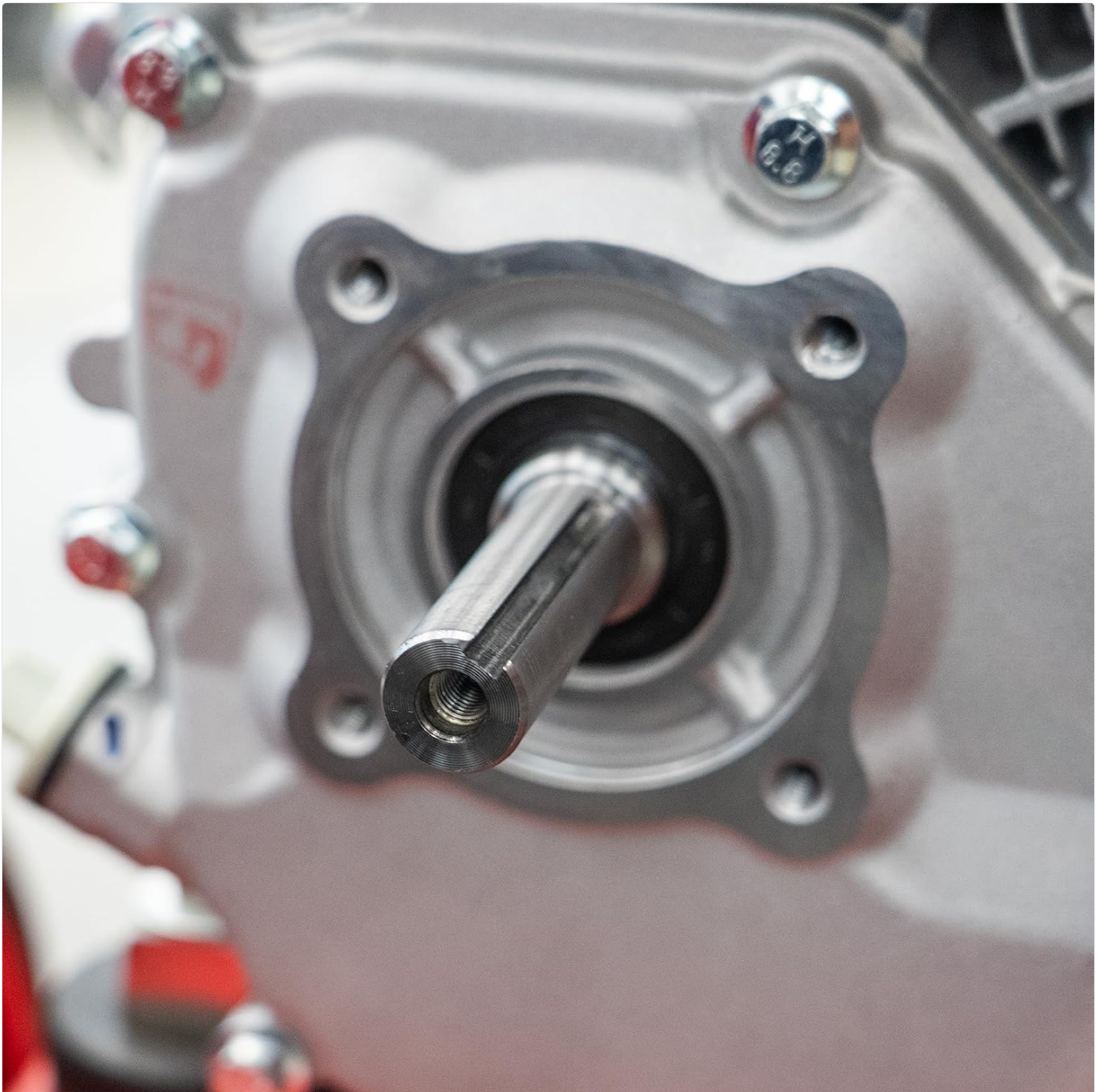
Image 5: A close-up view of the 3/4" horizontal shaft, illustrating the keyway and threaded end for secure pump attachment.
